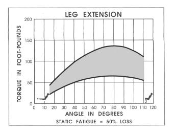
Again, with the third chart, we have two tests of fullrange strength; but in this case we are showing tests of static (isometric) strength. The highest curve shows the level of fresh strength, while the lower curve shows remaining strength following the exercise. The shaded area between the two curves shows fatigue produced by the exercise. Fresh static strength had been reduced by 50 percent.
